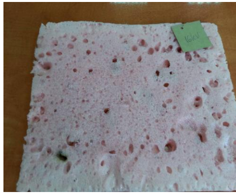
FIGURE 4 - FIREPROOF MATERIAL – EXPANDED POLYURETHANE FOAM
